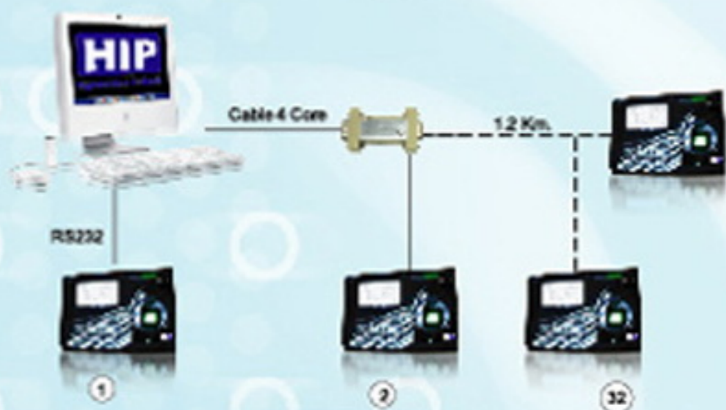
Connection Type Series RS232 and RS485
